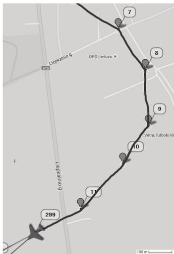
To eliminate problems after sharp turns, loops around the turns were created [10]. As seen in Fig. 8, placing one way-point 50 meters behind a sharp turn (way-point 5) was not enough to make the aircraft return to the course correctly. Creating a circle of way-points (wp. 10-17) with radius of about 50 meters after a sharp turn turned out to be enough to make the UAV return to the intended path at a correct angle.
