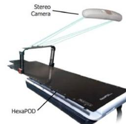
Fig. 1 System Setup
